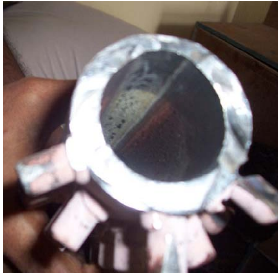
Photo 1- shows the deposition of chemical at top portion of bed tube.
