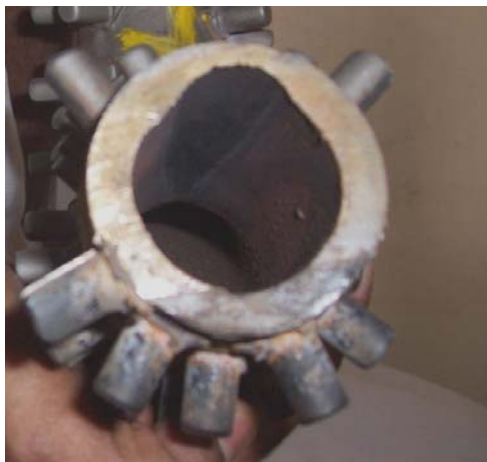
Photo 2- shows the material loss at top portion of bed tube.
